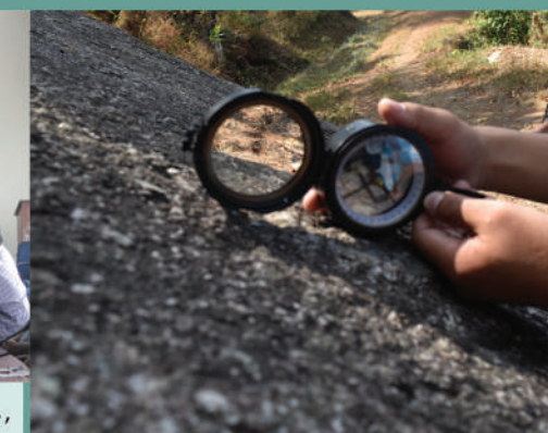
Calculating the Strike and Dip of a rock using a Clinometer and a Brunton Compass. This is required to identify the recharge area of a spring for rejuvenation.
