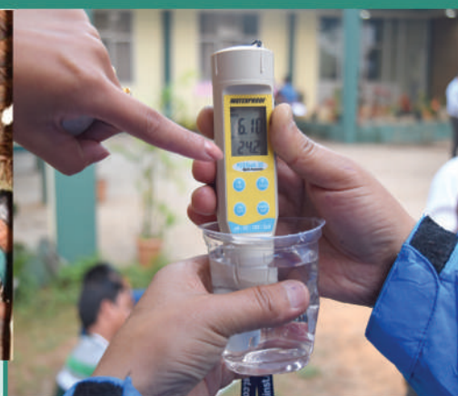
Water Quality Testing using a Water Tracer. Water temperature, Salinity, PH, TDS and Alkalinity are the parameters tested.
